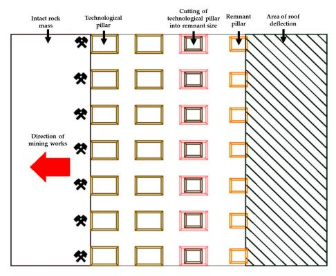
generate conditions that *favor* the softening and yielding of the floor and pillars and result in the accumulation of elastic energy above the mining area.
