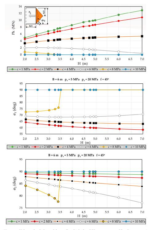
**Figure 7.** Values of unbalanced forces  $P_k$  which should be compensated by the appropriate ground support system (**top**), angle  $\alpha_2$  (**middle**), and angle  $\alpha_1$  (**bottom**), assessed for a specific case of excavation geometry, load, and strength characteristics of surrounding rocks.
