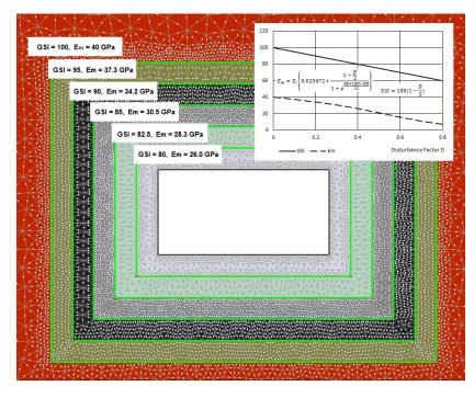
**Figure 8.** Modulus of deformation of surrounding rock mass, scaled down using the Hoek–Diederichs approach [41].
