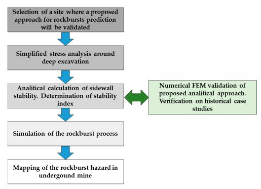
Figure 3. General flowchart diagram explaining the proposed methodology.
