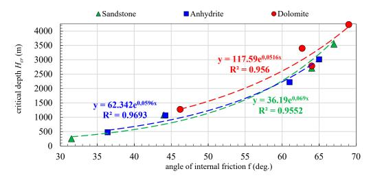
**Figure 12.** Critical depth for different types of rocks within a drift's sidewall in selected mininggeologic conditions (B = 6 m, H = 3 m,  $p_x = 10 \text{ MPa}$ ).
