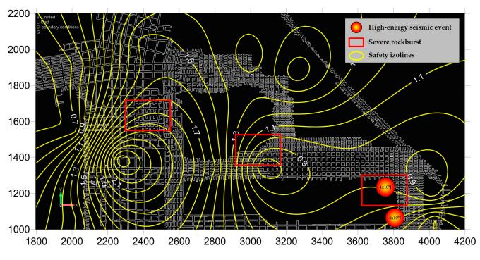
Figure 13. Rockburst safety factor distribution over one of the analyzed regions in the Rudna mine.
