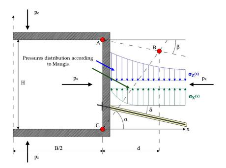
**Figure 4.** Physical model of the sidewall loading for the case of a deep opening excavated within a homogeneous or joined rock mass.
