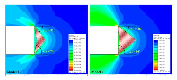
Figure 9. Maximum shear strain distribution obtained numerically (model 1, top; model 4, bottom).
