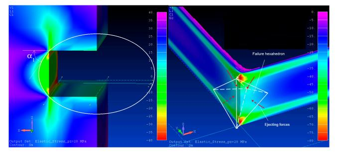
**Figure 10.** Quarter of the entire intersection; contour of the values of safety margin within sidewalls of the gallery (**left**); contours of slip planes of the failure hexahedron at the underground galleries' intersection (**right**).
